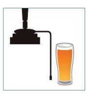
Allow to settle. Top-up as necessary, keeping sparkler below head. Aim for a 10mm deep head.
